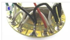
Some solder joints will span two pads - place the link wire between both pads and run the solder onto both pads evenly.
