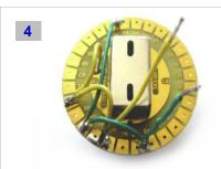
Solder the link wires onto the numbered pads as shown. Do not pre-tin the pads and avoid using excessive solder. Note ground connection.
