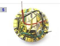
Link wire soldering completed - the wiring should not protrude beyond the switch perimeter to facilitate clean install.
