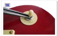
Screw the toggle tip tightly onto the threaded shaft - the pliars will prevent the shaft from rotating.
